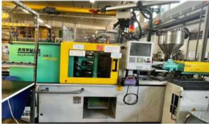
INJECTION MACHINE #7 : ARBURG 50T - A321
