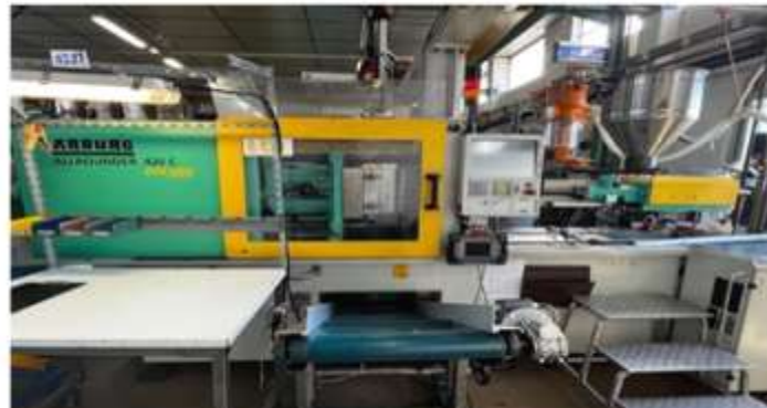
INJECTION MACHINE #5 : ARBURG 100T- A420
